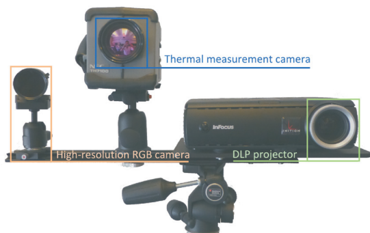
Figure 2. Configuration of the static 3D thermal imaging component. The component consists of a high-resolution RGB camera, a DLP projector and a thermal measurement camera.
