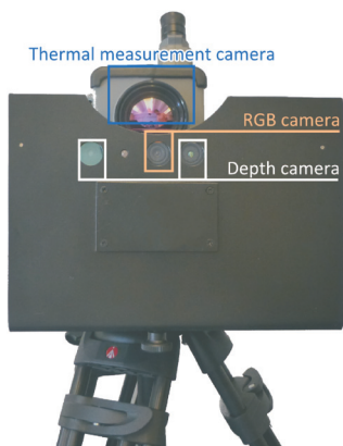
Figure 3. Configuration of the dynamic 3D thermal imaging component. The component consists of a RGB camera, a depth camera and a thermal measurement camera.
