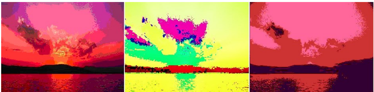
Figure 11. Original color image (left) vs. segmented image under mean-shift (middle) vs. segmented image under SMEB (right) for sunset image
