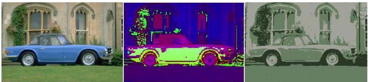
Figure 10. Original color image (left) vs. segmented image under mean-shift (middle) vs. segmented image under SMEB (right) for car image
