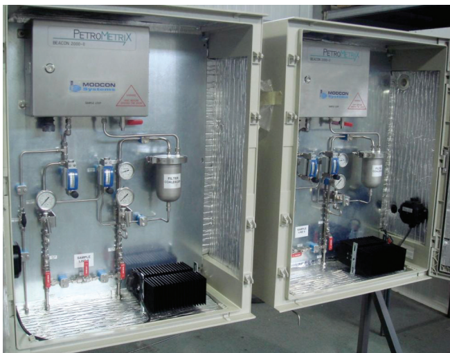
Slika 2 – Procesni NIR analizator (Process NIR Analyser) 6
