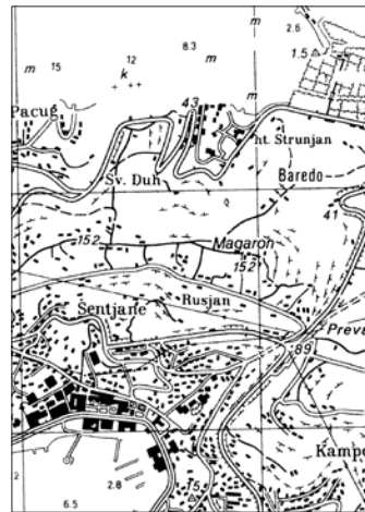
Figure 2. black color, V layer, buildings, names printed with V colorants with a composition that does not absorb the NIR light (R,G,B = 0%, 0%, 0% ; C,M,Y,= 33%, 33%, 33%)
