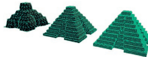
Figure 14. Level of detail (LD), from left LD=2, LD=5, LD=10.
