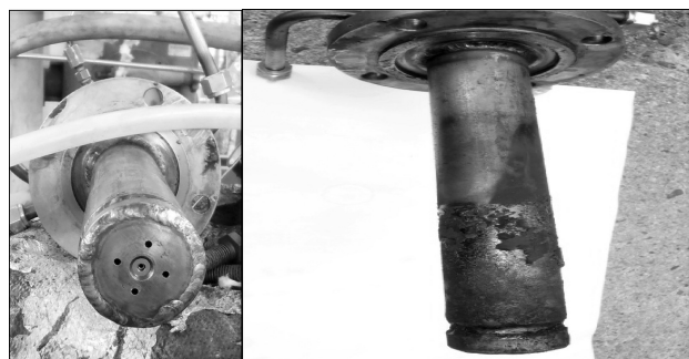
Fig. 1 – Nozzle of pilot plant reactor before (left) and after (right) experimental test
