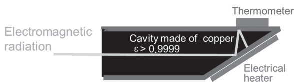
Fig. 2: Schematic of an electrical substitution radiometer [1]
