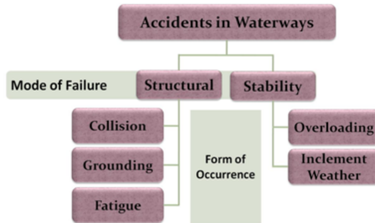
Fig. 5 Mode of failure and form of occurrence of accidents in waterways
