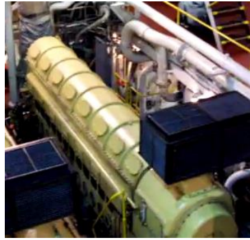
Fig. 1 Fairbanks-Morse 38D8-1/8 installed on a submarine
