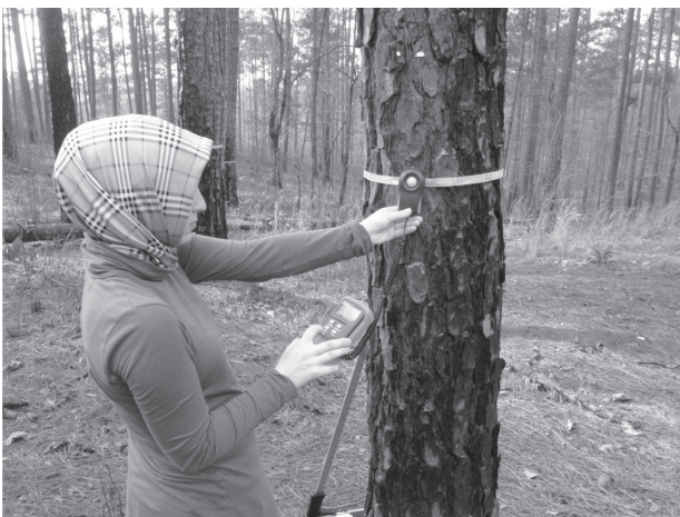
Fig. 3 Light conditions being measured using the Mastech LX1330B light meter
