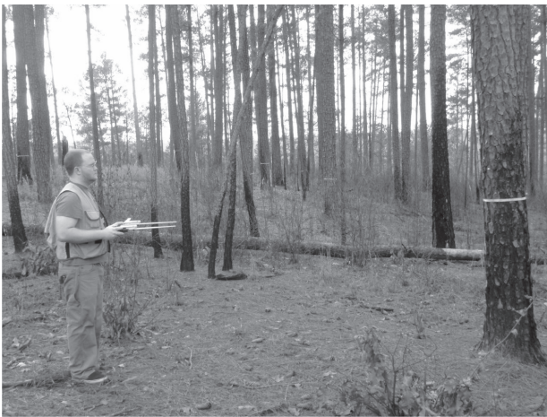
Fig. 2 Remote measurements conducted with the laser caliper dendrometer
