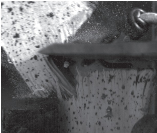
Fig. 10 Wood fiber failure during the second stage
