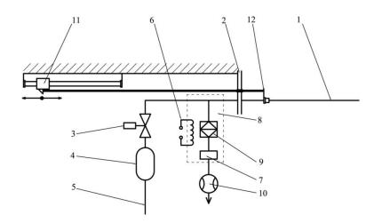
**Figure 1.** Scheme of the entire  $O_2$  analyser. 1 – extraction pipe, 2 - connection port, 3 – electromagnetic valve, 4 - air storage vessel, 5 - connection to the compressed air line, 6 – PID controlled heater, 7 -  $\lambda$ -sensor, 8 - isolated box, 9 – filter, 10 – air pump, 11- linear drive unit, 12 – slag scraper
