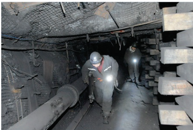
Figure 9 Severe roof-to-floor convergence in the cut-through entry at which conventional wood cribs were installed
