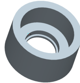
Figure 1. Three dimensional solid model of the bearing sleeve.
