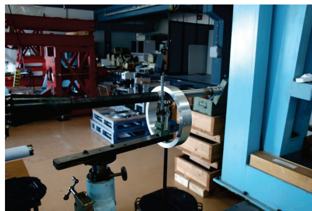
Figure 9 Sting deflection and slope measurement
