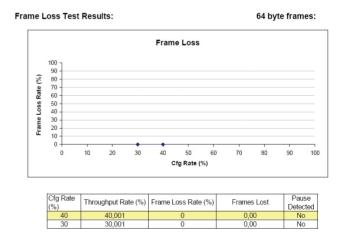
Fig. 9 Testing frame loss ratio of Ethernet link with 64 bytes frame length (test: pass) Slika 9. Ispitivanje učestalosti gubitka okvira Ethernet veze s
