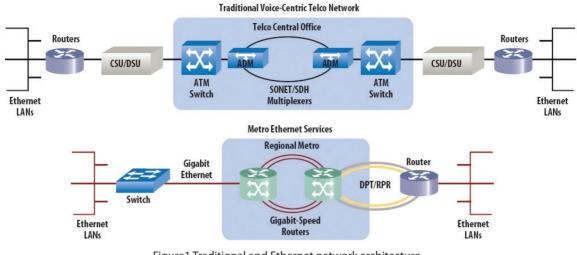
Figure1 Traditional and Ethernet network architecture Slika 1. Arhitektura tradicionalne i Ethernet mreže
