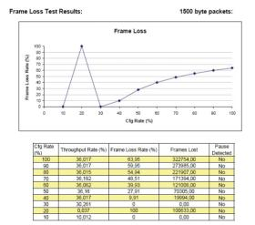
Fig. 12 Testing frame loss ratio of Ethernet link with 1500 bytes frame length (test: fail)
