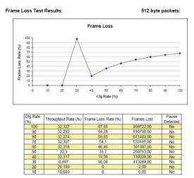
Fig. 10 Testing frame loss ratio of Ethernet link with 512 bytes frame length (test: fail)
