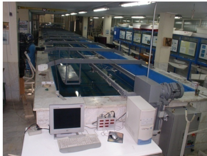
Fig. 5 Towing tank facilities of the Marine Research Centre (MRC) at the Sharif University of Technology (SUT)
