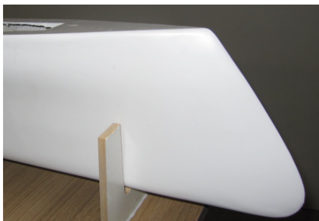
Fig. 1 Wave piercing bow profile of the centre hull (main hull)
