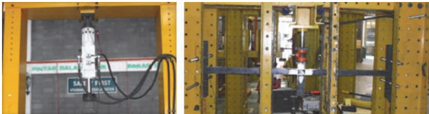
Figure 6. Dynamic actuator and hydraulic jack used for seismic and progressive collapse evaluations
