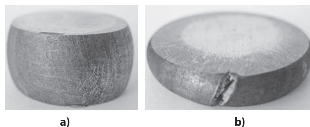
Figure 6 View of the specimens after the cold upsetting process: a) upsetting up to the 2/3 of the initial height; b) upsetting up to the 1/3 of the initial height
