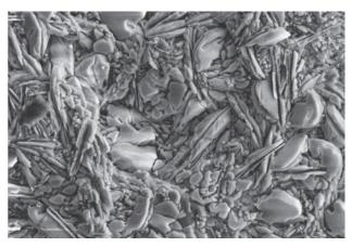
Figure 3 Structure of the two-phase phosphate layer, magnification 500 x
