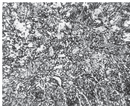
Figure 6 Filler material – sample 2, attack with Nital 2 / %; 100 ×
