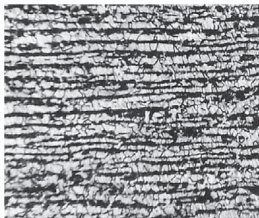
Figure 5 Base material – sample 2, attack with Nital 2 / %; 100 ×
