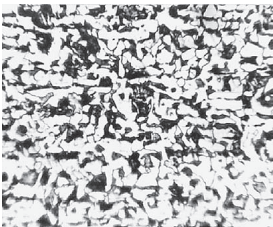
Figure 2 Base material – sample 1, attack with Nital 2 / %; 100 ×
