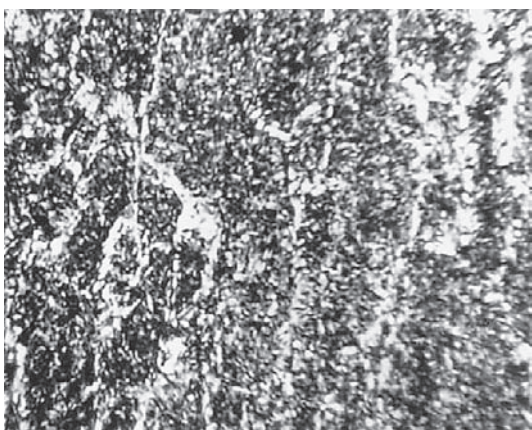
Figure 3 Filler material – sample 1, attack with Nital 2 / %; 100 ×
