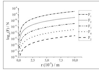
**Figure 2** The frictional force  $F_d$  for a single SiC particle in the vicinity of a vertical solidification front, which is advancing horizontally, for the particle velocities  $V_p = 10^{-6}$  /m s<sup>-1</sup> (ZnAl8/SiC<sub>p</sub>)
