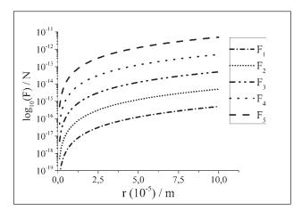
Figure 9 The Saffman forces for ZA27/SiC  $_{\rm p}$  composite (S=0,000001 /m s^-1)
