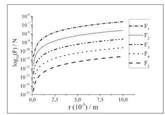
**Figure 7** The frictional force  $F_d$  for a single SiC particle in the vicinity of a vertical solidification front, which is advancing horizontally, for the particle velocities  $V_p = 10^4 / \text{m s}^{-1}$ , (ZnAl27/SiC<sub>p</sub>)
