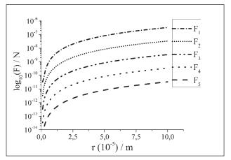
**Figure 4** The frictional force  $F_d$  for a single SiC particle in the vicinity of a vertical solidification front, which is advancing horizontally, for the particle velocities Vp=  $10^{-4}$  /m s (ZnAl8/SiC<sub>n</sub>)
