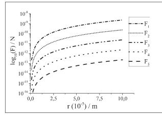
**Figure 5** The frictional force  $F_d$  for a single SiC particle in the vicinity of a vertical solidification front, which is advancing horizontally, for the particle velocities  $V_p = 10^{-6} / \text{m s}^{-1} (\text{ZnAl27/SiC}_p)$
