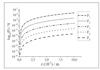
**Figure 6** The frictional force  $F_d$  for a single SiC particle in the vicinity of a vertical solidification front, which is advancing horizontally, for the particle velocities  $V_p = 10^{-5} / \text{m s}^{-1} (\text{ZnAl27/SiCp})$
