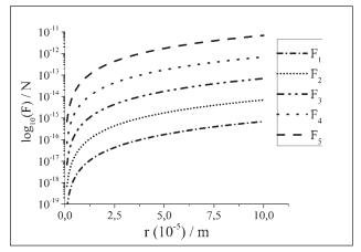
Figure 8 The Saffman forces for ZA8/SiCp composite. (S=0,000001 /m s<sup>-1</sup>)
