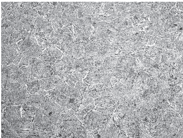
Figure 2 Microstructure of the heat affected zone (100x)
