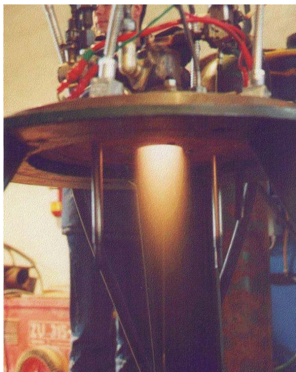
Figure 5. Formation of the oxygen-hydrogen flame Slika 5. Formiranje plamena kisika i vodika
