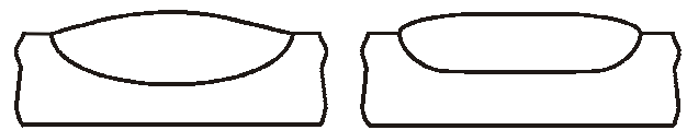
Figure 5. Shape of the surfacing weld as a function of the arrangement of wires of different diameters
