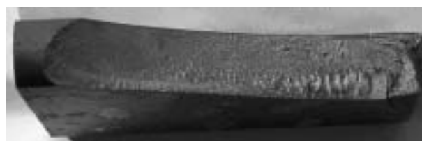
Figure 1. Brittle cracking of rolled profiles in mechanical cutting due to remaining internal hydrogen
