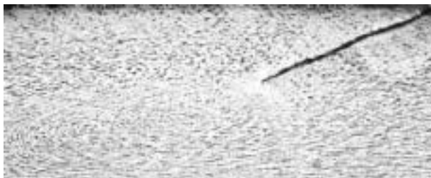
Slika 11. Prevaljanost na pilgeru -jednostruka Figure 11. Overlapped state - single - in pilger mill
