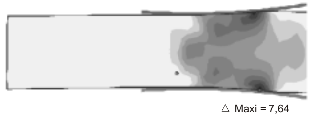
Figure 4. Distribution of stresses \sigma_y within the roll gap, with h_0 = 105,76 mm, \epsilon = 10\% , \theta = 2^\circ
