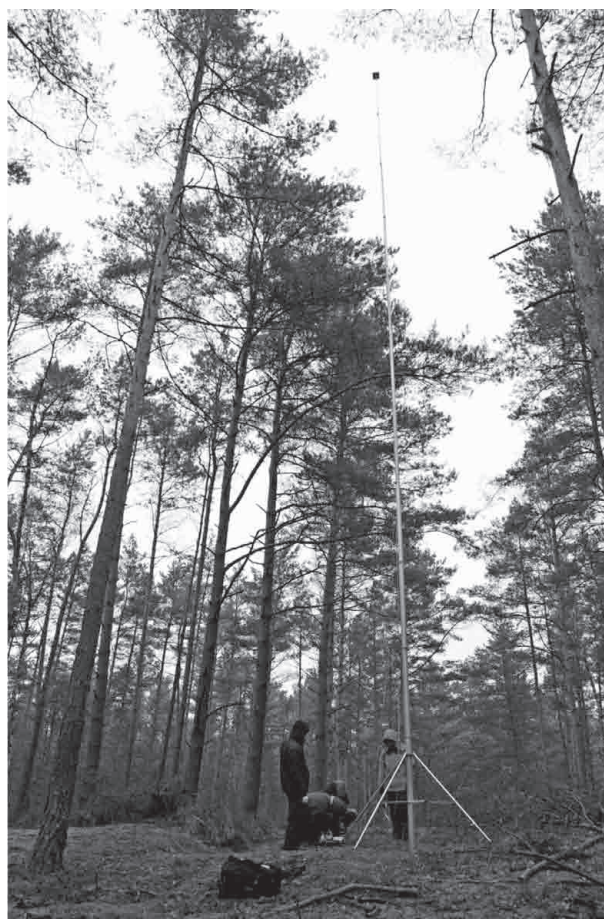
Fig. 1 An aluminum telescopic mast with the GNSS receiver in the Głuchów forest district (photo: Dariusz Górscy)
