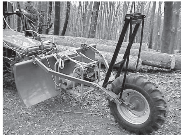
Fig. 5 The fifth wheel used on the front part of the tractor
