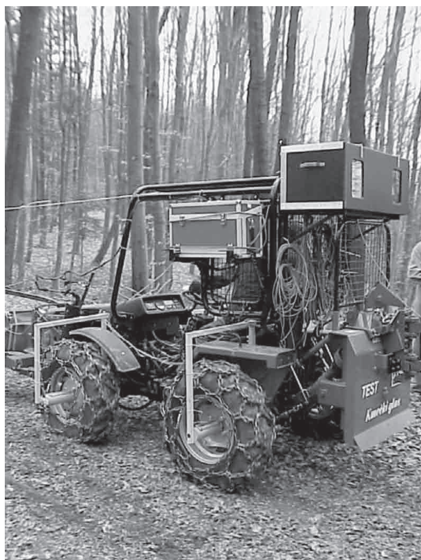
Fig. 2 Adapted agricultural tractor AGT 835 T with measurement equipment
