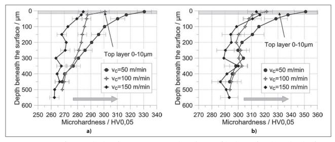
**Figure 1** Comparison of DSS microhardness for various cutting speeds as a function of the distance from the machined surface measured for the grains of ferrite (a) and austenite (b) ( $f = 0,3 \text{ mm/rev}, a_n = 2 \text{ mm}$ )
