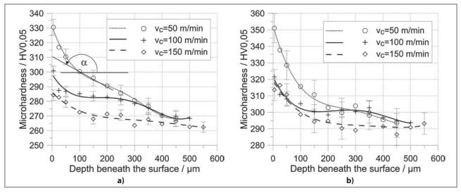
Figure 2 The course of functions approximating the sets of microhardness change points as a function of the distance from the material surface for various cutting speeds for ferrite (a) and for austenite (b) with f = 0.3 mm/rev,  $a_n = 2$  mm
