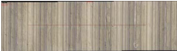
Fig. 1 Surface texture of a sample turned with the T1 tool point in real colour
