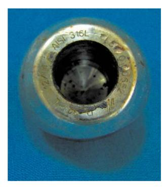
Fig. 3. Worn metal head type AISI 316L.
