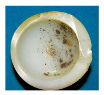
Fig. 5. Worn polyethylene insert with metal debris.
