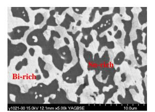
Figure 2. The microstructure of Sn58Bi.
