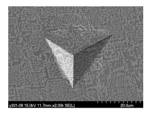
*Figure 5. SEM image of residual indent on solder alloy.*
