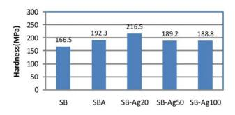
Figure 6. Hardness of solder alloys.
