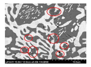
Figure 3. The microstructure of Sn57Bi1Ag.
