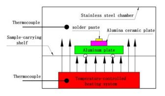
Figure 1. A schematic of the experimental device.
