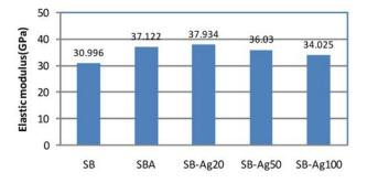
Figure 7. Elastic modulus of solder alloys.
