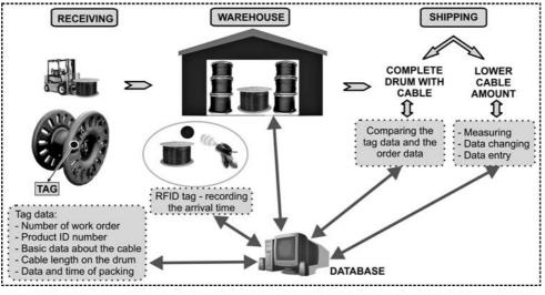
**Figure 4** The application of RFID technology in cable storage
