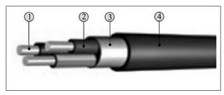
Figure 1 Product composition: 1 – Cu conductor, 2 – PVC insulation, 3 – unvulcanized tire filling and 4 – PVC sheath
