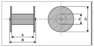
Figure 2 Design features of drums: B – drum width, b – traverse width, D – drum diameter and d – traverse diameter
