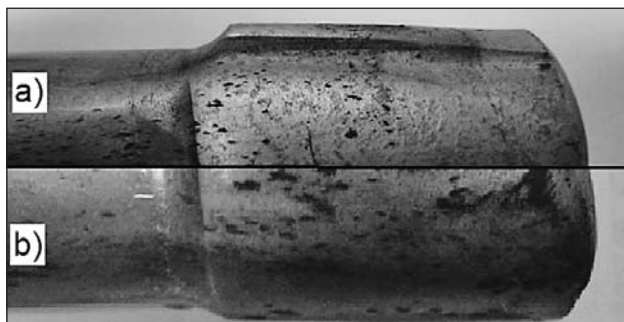
Figure 4 End necks of preforms rolled after billet heating: a) 20 minutes, b) 40 minutes
