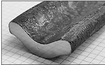
Figure 6 The view strands after rolling in a steel sample after the third groove
