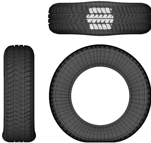
Figure 6. Deformed shape of detailed tread model, inflated to 2 bars, under vertical load F_z = 3580 N, with footprint contact pressure shown
