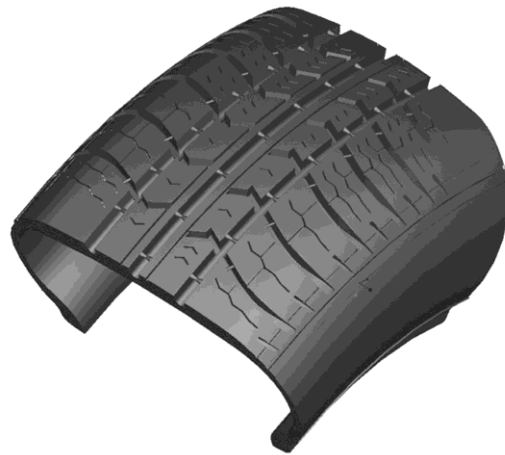
Figure 1. 3D parametric model of an existing tire type, dimensioned 165/70R13
