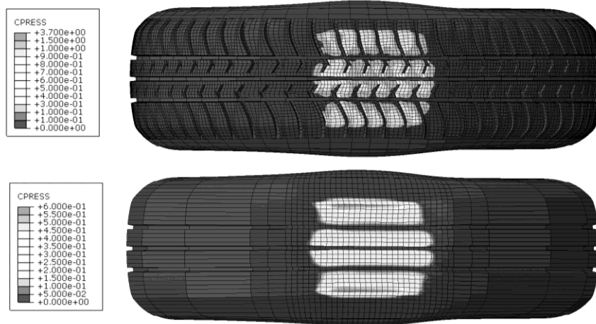
Figure 9. Comparison of contact pressure obtained using simplified and detailed tread models, at full braking
