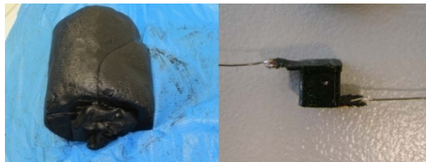
Figure 5. Raw conductive silicone rubber Elastosil R570/70 and one cubic sensor-specimen
