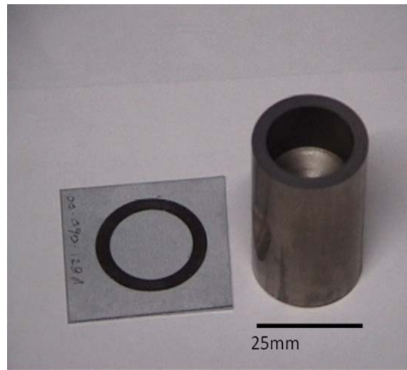
Figure 26: TCT test specimens - flat (left), annular (right)
