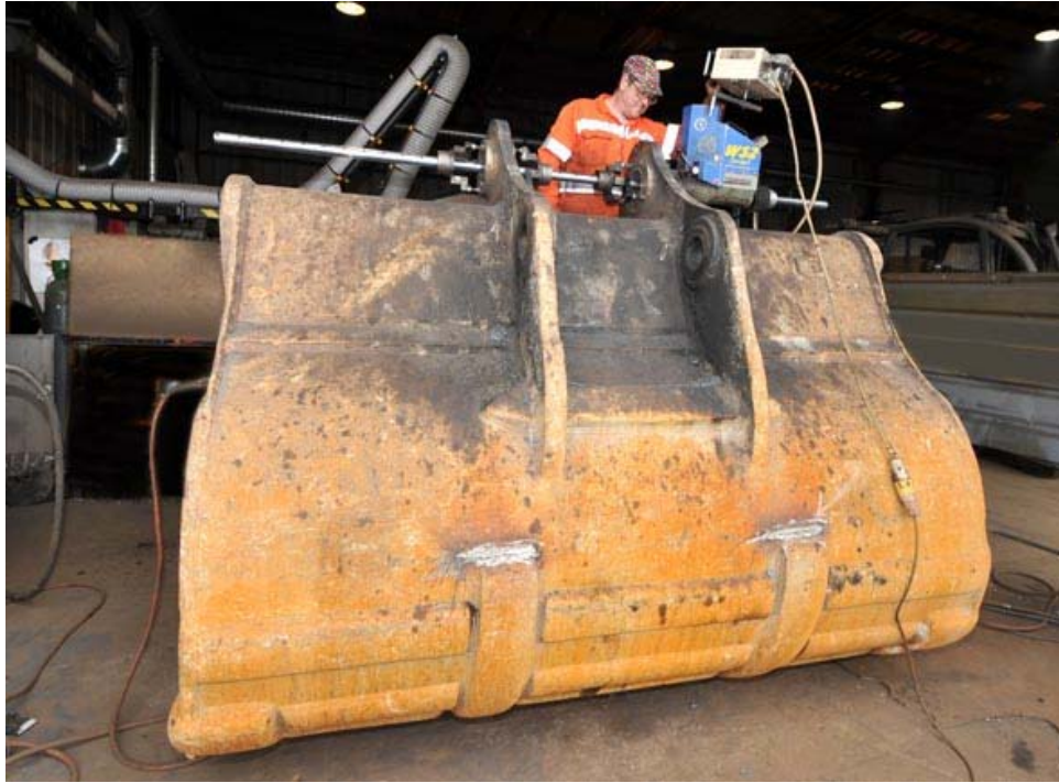
Figure 3: Catastrophic adhesive failure of a scoop bucket pivot bushings necessitates rebuilding of the bucket pivots with mobile line-boring equipment. [15]
