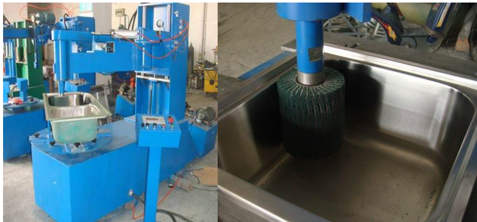
Figure 62: Grinding of the inside of a deep drawn stainless steel sink [102]
