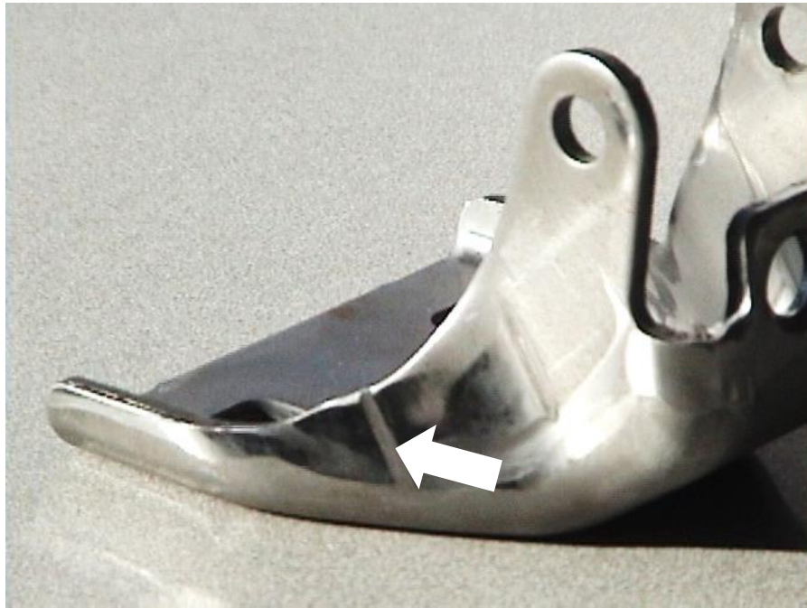
Figure 6: Galling of a truck door hinge rendering the part unusable. The white arrow indicates severe adhesive wear (galling) affecting part quality.
