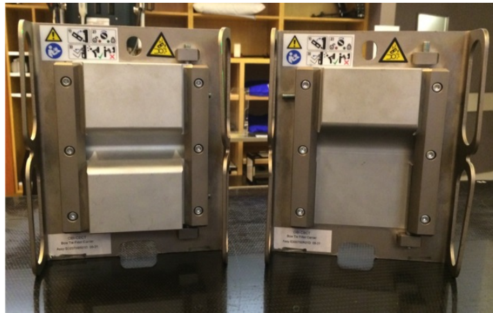
Figure 4.2: Full and half bow-tie filter used in the OBI imaging system.
