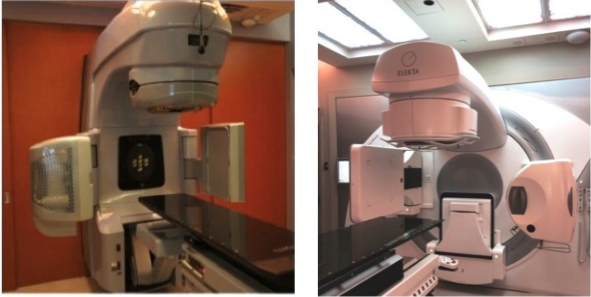
Figure 4.1: The kV CBCT systems used in this study, left: the Varian OBI, right: Elekta XVI.*
