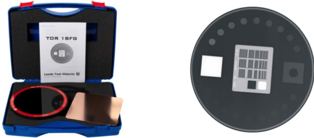
Figure 4.6: The TOR 18FG Leeds phantom (left) and its kV planar image (right). High contrast resolution and low contrast sensitivity modules are located in the central and peripheral region of the phantom, respectively. 46
