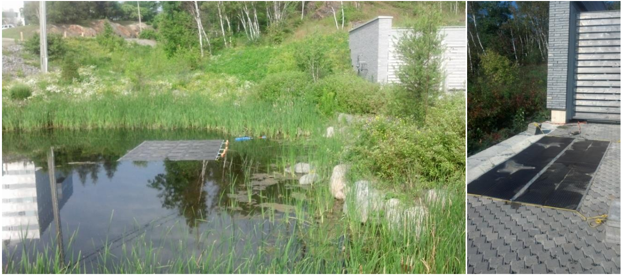
Figure 2-7: MIRARCO's Floating PV Prototype (Left) and the control ground mounted nearby panels (Right) – Sudbury, Canada
