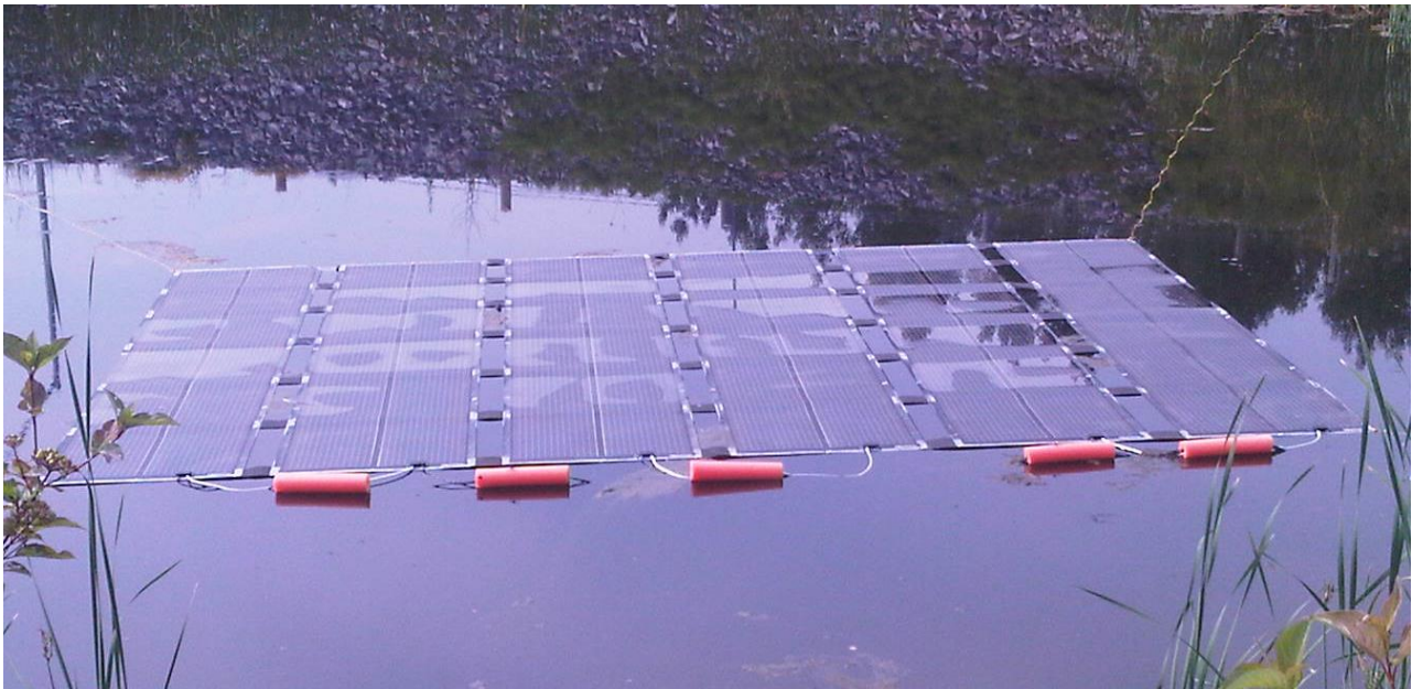
Figure 5-1: Floating thin film PV array prototype in Sudbury, Canada
