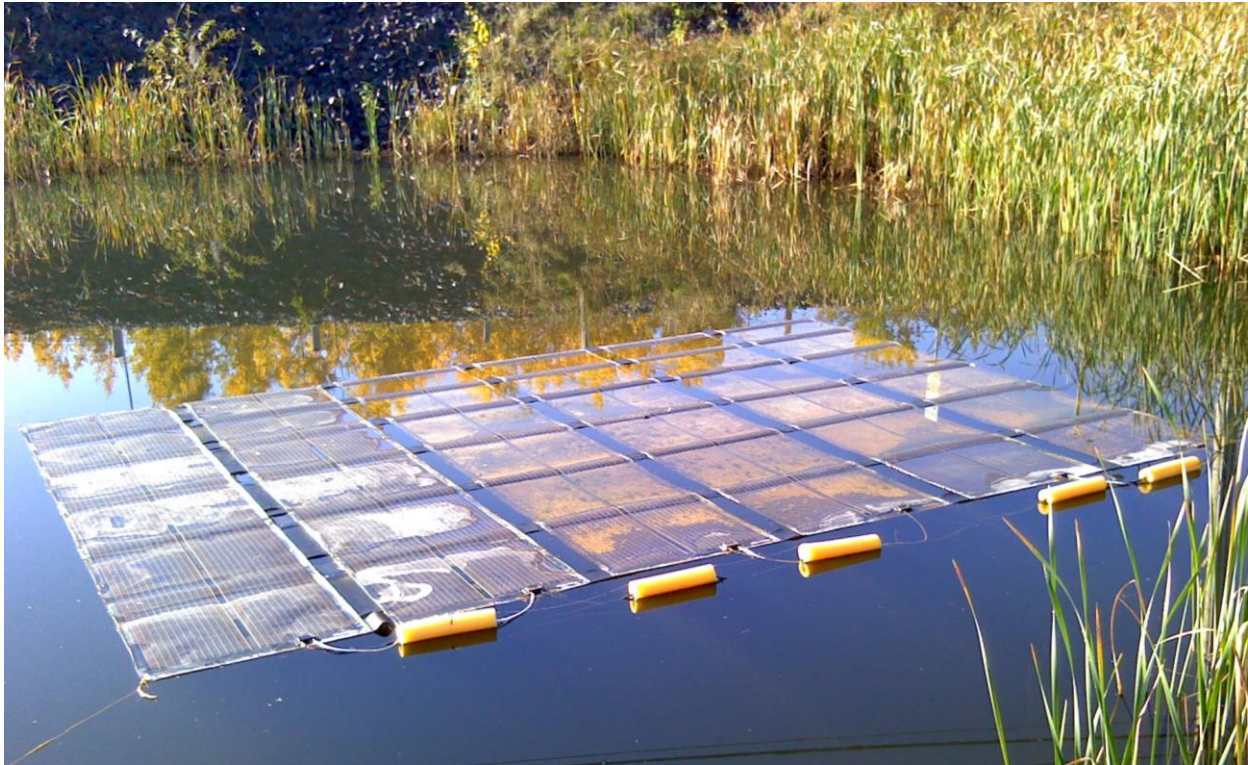
Figure 10-2: Floating PV array with 4 panels on right operating under a cm of water after a 4 month deployment
