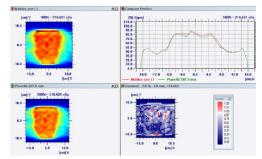
Figure 3 demonstrates the plan verification of an IMRT plan (FFF) calculated for one machine and treated at the other. The gamma image was evaluated with 3% and 3mm and passed with 97% of pixels in range.
