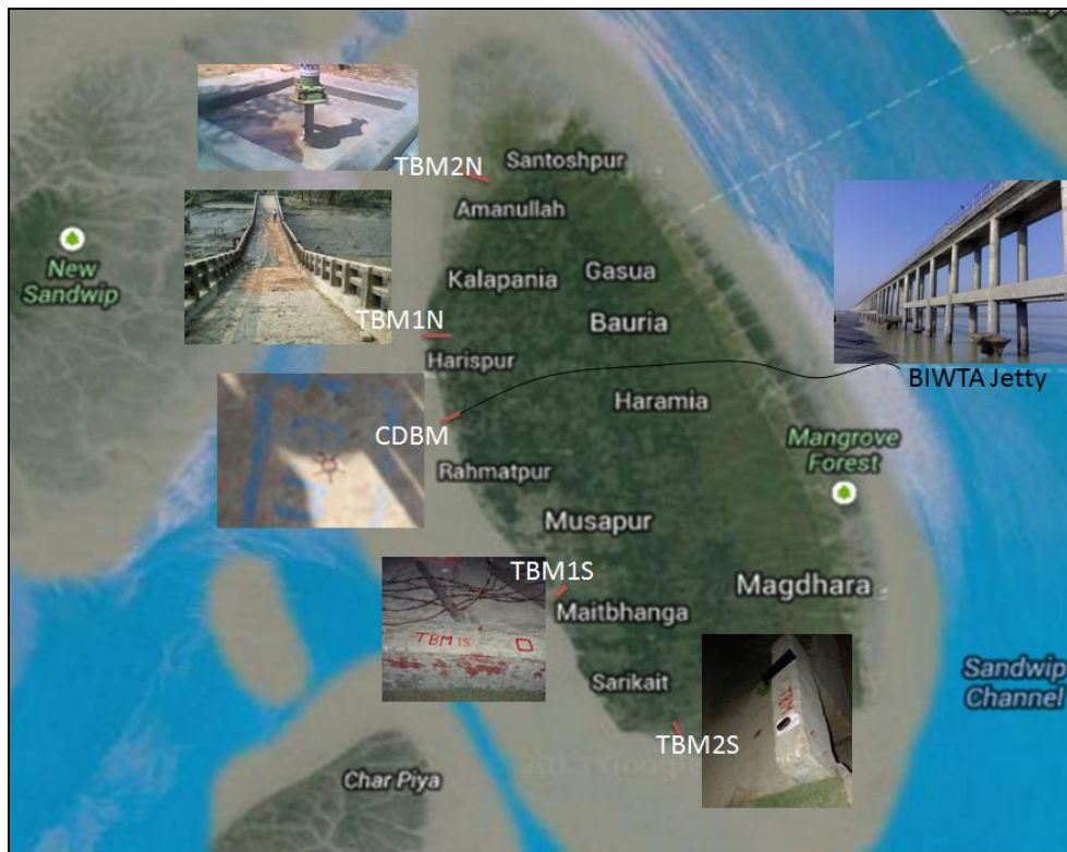
Figure 3. 8: Photo of TBM established structure location in Sandwip by total station
