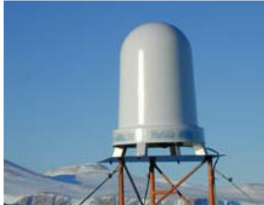
Figure 2.1: The external dome-shaped device of Pludix in which are housed the active sensors of the instrument.
