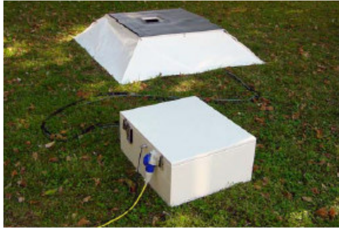
Figure 2.7: The Sensor Unit and the Outdoor Electronics Unit of the 2DVD. Schonuber (2007).
