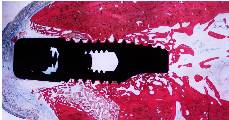
Figure 17: histological slides were thinned to about 50 \mu\text{m} and stained with Stevenel's blue with alizarin red
