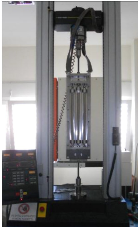
Figure 70 Experimental setup for the testing of the new proposed SMA device. University of Ferrara.
