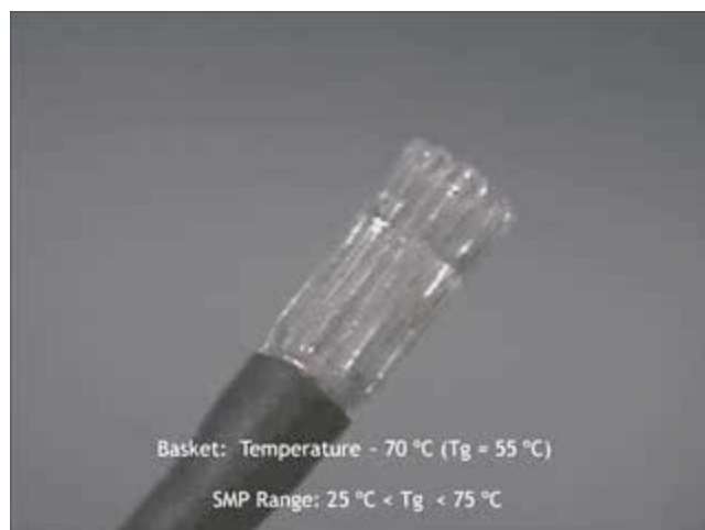
Figure 46 Basket for catching large emboli (micro-injection molded).
