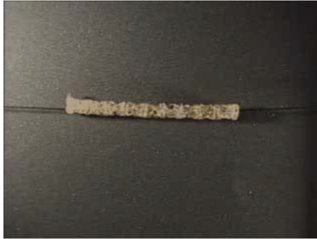
Figure 44 SMP stent, dip coated and laser machined.
