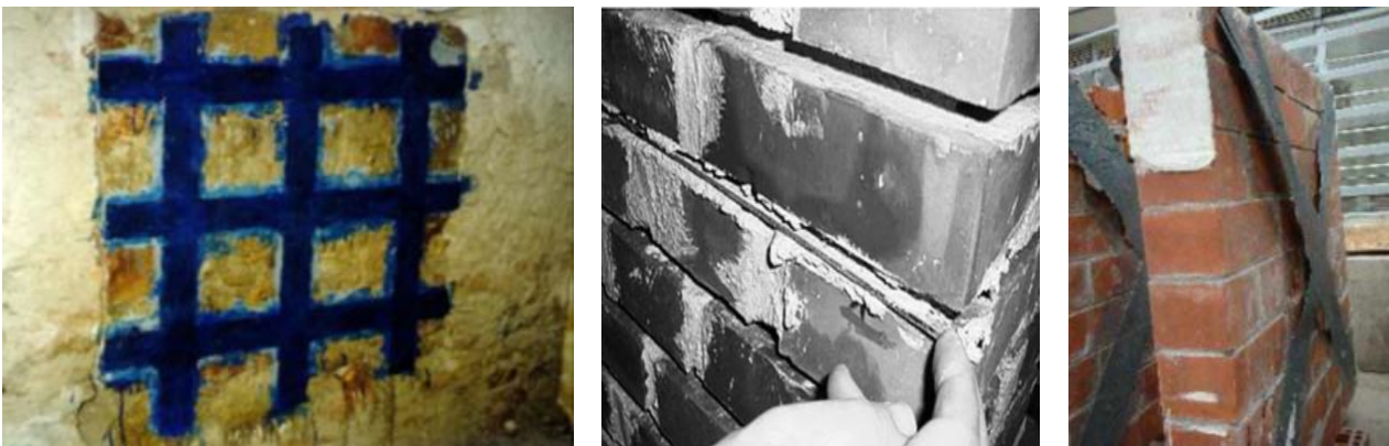
Figure 62 Examples of different CFRP reinforcement during tests on masonry specimens: (a) panel strengthened with CFRP strips (Borri et al., 2001); (b) creep simulation on sample strengthened with thin CFRP strips (Valluzzi, 2007); (c) CFRP fabric debonded after failure (Santa Maria et al., 2004).
