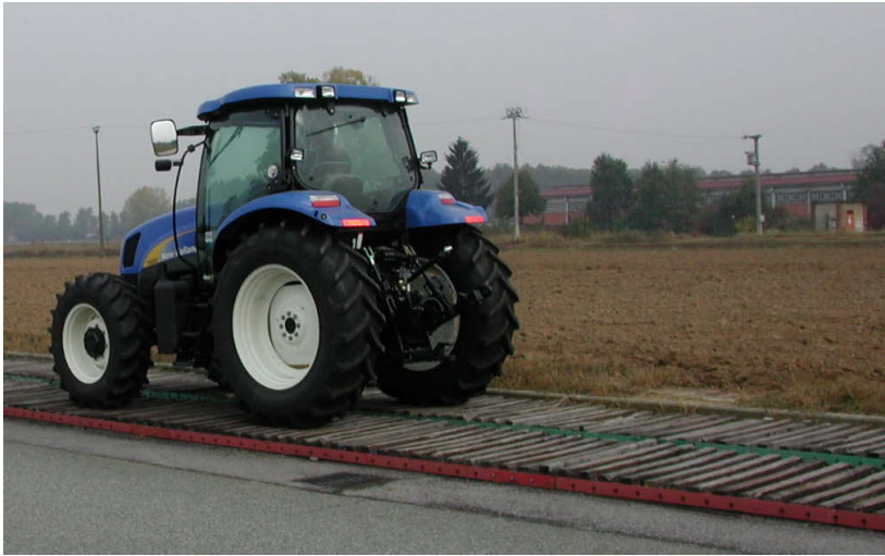
Figure 30. Smooth artificial test track, compliant with ISO 5008 International Standard [50].
