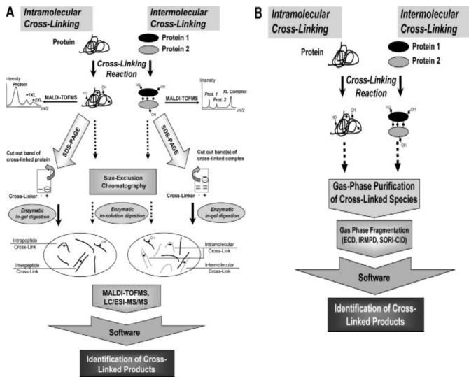
General analytical strategies for protein structure characterization by chemical cross-linking and mass spectrometry. (A) Bottom-up approach, and (B) top-down approach using FTICR-MS.
