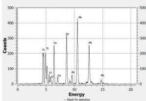
**FIG. 63** PIXE spectra of red-white pigment, low energy detector. Experimental set up: particle/energy 3 MeV, current p+, Dose/s 200 50 KeV, Helium flow.
