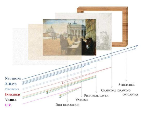
**FIG. 8** Schematic representation of the different penetration depth and layers probed by various analytical techniques that employ diverse radiation and particle source<sup>6</sup>.
