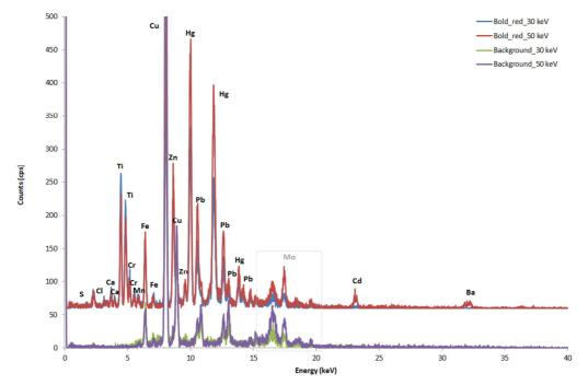
**FIG. 132** XRF spectra on red sample: total spectra from different set-up, not subtracting background. Experimental set up: voltage 50 KeV and current 700  $\mu$ A, voltage 30 KeV and current 1300  $\mu$ A. Live time: 60 s, no filter, Helium flow, Anode Molybdenum, collimator 0.200  $\mu$ m.
