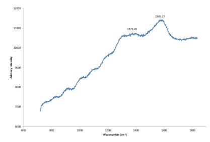
FIG. 47 Raman spectra on dark-brown particles (632,81 nm excitation, 50 x magnification): carbon (Black lamp pigment).
