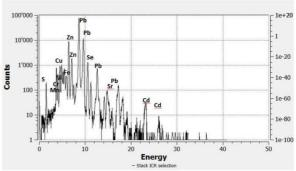
**FIG. 127** PIXE spectra of white behind, high energy detector.
