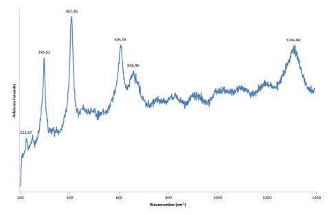
FIG. 68 Raman spectra on red-orange pigment (632,81 nm excitation, 2 mW, 30 s acquisition time): Hematite phase.
