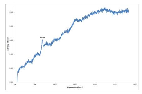
**FIG. 130** Raman spectra on white sample (632,81 nm excitation, 2 mW, 50 s acquisition time): High fluorescence, Barium Sulphate peak at  $984 \text{ cm}^{-1}$ .
