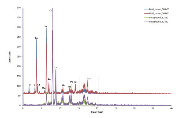
**FIG. 123** EDXRF spectra on the backside of White sample: total spectra from different set-up, not subtracting background. Experimental set up: voltage 50 KeV and current 700  $\mu$ A, voltage 30 KeV and current 1300  $\mu$ A. Live time: 60 s, no filter, Helium flow, Anode Molybdenum, collimator 0.200.
