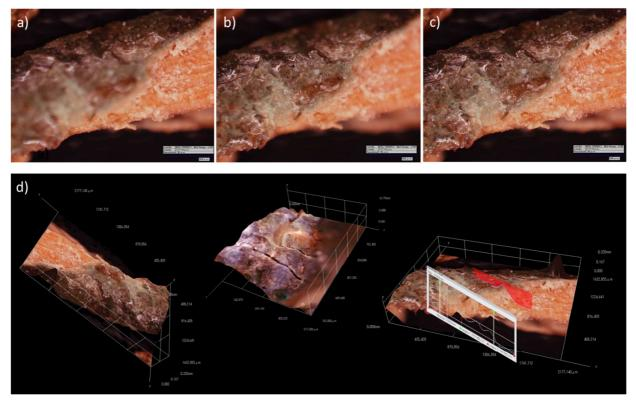
**FIG. 17** 3D Digital Microscope System Hirox KH-7700 (CNRS-LC2RMF UMR 171, Palais du Louvre - Paris, France): a) microphotograph of sample, focused on wood support (magnification 140 X); b) microphotograph of studied sample, focused on pictorial layer (magnification 140 X); c) microphotograph of studied sample, obtained by multi-focus system; d) 3D model of sample in the previous image and surface profile measurements.
