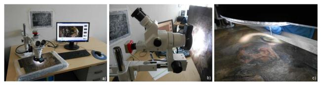
**FIG. 16** Stereomicroscope OPTIKA SZ6745TR (Physics and Earth Science Department, Ferrara University, Italy): a) horizontal working set up; b) vertical working set up; c) sampling on artwork "Reader woman on bed and old man" (artwork plate IV) under stereomicroscope.
