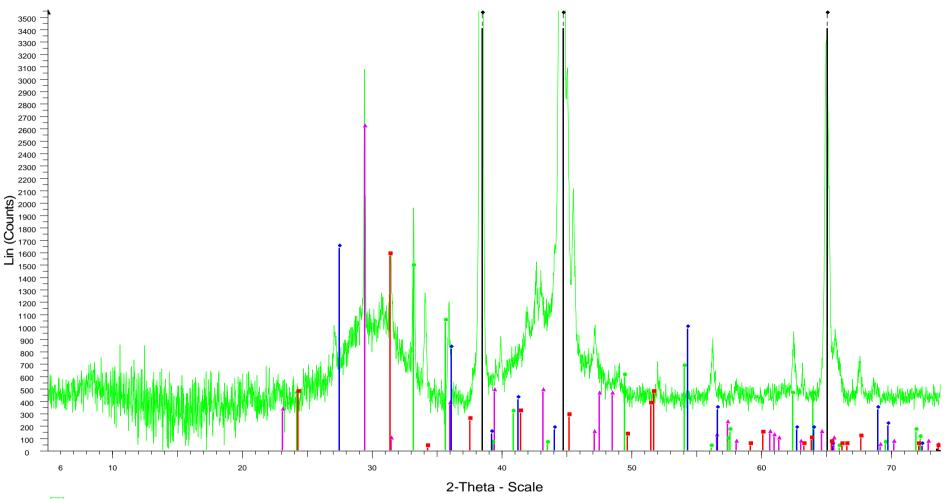
PIC (L.Volpe) - Al stub - plexi - File: Prova-PIC\_Al-stub\_plexi.raw - Type: Locked Coupled - Start: 5.000 ° - End: 80.000 ° - Step: 0.020 ° - Step time: 15. s - Temp.: 25 °C (
