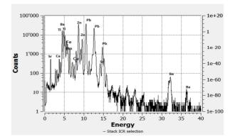
**FIG. 60** PIXE spectra of white pigment, high energy detector. Experimental set up: particle/energy 3 MeV, current p+, Dose/s 200 50 KeV, Helium flow.
