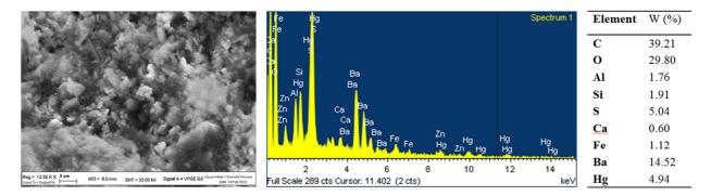
FIG. 135 SEM/EDS analysis on red sample.
