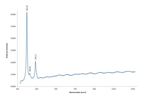
**FIG. 79** Raman spectra on red sample (632,81 nm excitation, 2 mW, 50 s acquisition time):Vermilion. Source: Ferrara University.
