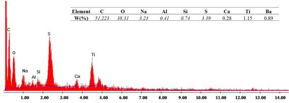
FIG. 55 EDS spectra and analytical data of pigment: results of average measure carried out in different point on white samples. In italic, average value greater than  $\sigma$ .
