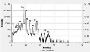
**FIG. 125** PIXE spectra of white pigment, high energy detector.
