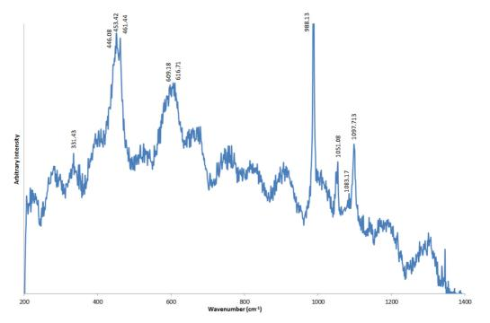
**FIG. 67** Raman spectra on white pigment (632,81 nm excitation, 2 mW, 40 s acquisition time): rutile, calcite, barium sulfate, lead oxide.
