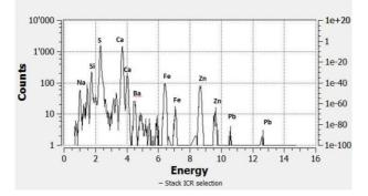
FIG. 126 PIXE spectra of white behind, low energy detector.
