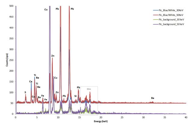
FIG. 58 XRF spectra on blue/white pigment: total spectra from different set-up, not subtracting background. Experimental set up: voltage 50 KeV and current 700  $\mu$ A, voltage 30 KeV and current 1300  $\mu$ A. Live time: 60 s, no filter, Helium flow, Anode Molybdenum, collimator 0.200
