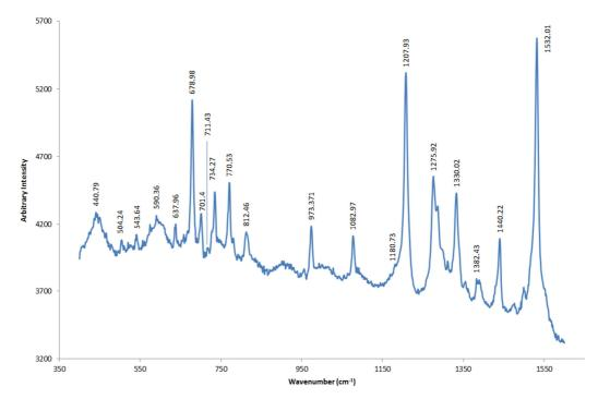
FIG. 48 Raman spectra on dark-brown particles (632,81 nm excitation, 50 x magnification): Burnt Green Earth.
