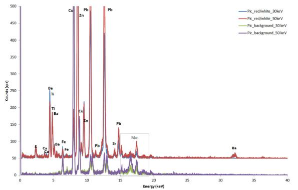
FIG. 57 XRF spectra on red/white pigment: total spectra from different set-up, not subtracting background. Experimental set up: voltage 50 KeV and current 700  $\mu$ A, voltage 30 KeV and current 1300  $\mu$ A. Live time: 60 s, no filter, Helium flow, Anode Molybdenum, collimator 0.200
