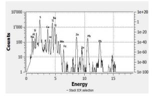
**FIG. 59** PIXE spectra of white pigment, low energy detector. Experimental set up: particle/energy 3 MeV, current p+, Dose/s 200 50 KeV, Helium flow.
