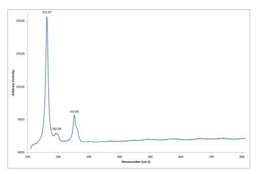
**FIG. 137** Raman spectra on other particle in red sample (632,81 nm excitation, 2 mW, 50 s acquisition time): Vermilion. Source: Ferrara University.
