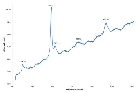
FIG. 80 Raman spectra on blue particles (632,81 nm excitation, 50 x magnification): Artificial Ultramarine Blue.
