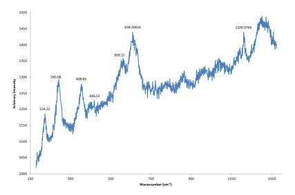
FIG. 46 Raman spectra on white-brown samples (632,81 nm excitation, 100 x magnification): Hematite and Rutile.
