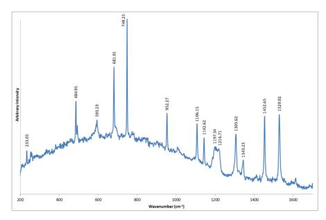
**FIG. 69** Raman spectra on Blue particle in white pigment (632,81 nm excitation, 2 mW, 50 s acquisition time): Phthalocyanine Blue.
