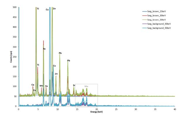
**FIG. 40** XRF spectra on Dark-Brown pigment: total spectra from different set-up, not subtracting background. Experimental set up: voltage 50 KeV and current 700  $\mu$ A, voltage 30 KeV and current 1300  $\mu$ A, 15 KeV and 1500  $\mu$ A current. Live time: 120 s, no filter, Anode Molybdenum, collimator 0.650.
