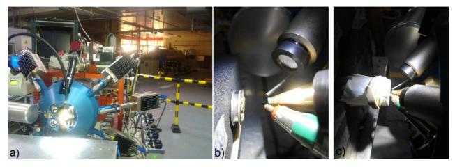
**FIG. 19** AGLAE facility (Centre de Recherche et de Restauration des Musées de France, Palais du Louvre, Paris – France): a) AGLAE, external microbeam used to perform PIXE analysis; b) PIXE analysis on samples placed on stub (specimens taken from studied Modigliani's artwork); c) PIXE analysis on free samples placed on filter in hand-made vacuum system (specimens taken from "Flowers" by F. De Pisis).
