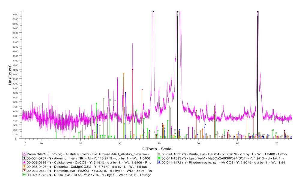
FIG. 49 XRD spectra obtained on stub containing white, brown and white/brown samples.
