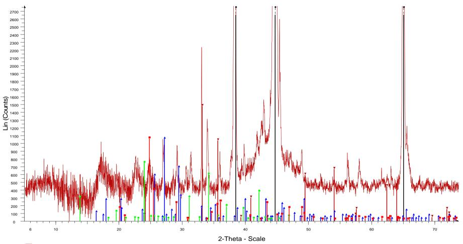
MOD (L.Volpi) - Al stub - plexi - File: Prova-MOD\_Al-stub\_plexi.raw - Type: Locked Coupled - Start: 5.000 ° - End: 80.000 ° - Step: 0.020 ° - Step time: 15. s - Temp.: 25 °
