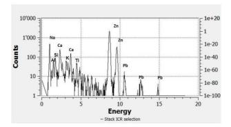
**FIG. 124** PIXE spectra of white pigment, low energy detector.
