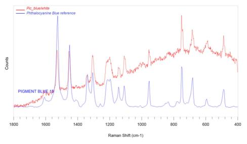
FIG. 70 Comparison Raman spectra obtained on analyzed sample (red) and Phthalocyanine Blue reference spectra.
