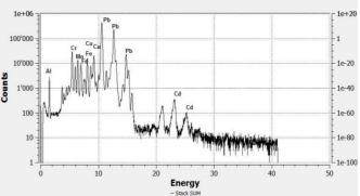
**FIG. 77** PIXE spectra of white pigment, low energy detector. Experimental set up: particle/energy 3 MeV, current p+, Dose/s 200 50 KeV, Helium flow.
