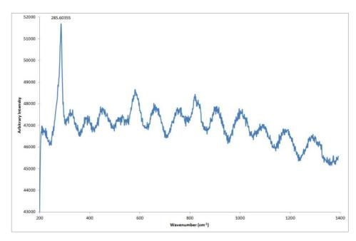
**FIG. 136** Raman spectra on red sample (632,81 nm excitation, 2 mW, 50 s acquisition time):Litharge. Source: Ferrara University.
