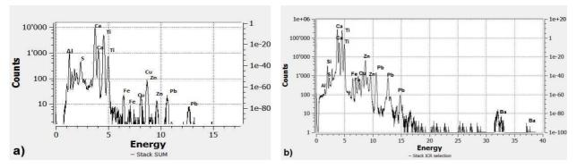
**FIG. 41** PIXE spectra of white pigment: a) low energy detector; b) high energy detector. Experimental set up: particle/energy 3 MeV, current p+, Dose/s 200, Helium flow.
