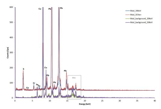
**FIG. 76** XRF spectra on White pigment: total spectra from different set-up, not subtracting background. Experimental set up: voltage 50 KeV and current 700  $\mu$ A, voltage 30 KeV and current 1300  $\mu$ A, Live time: 60 s, no filter, Anode Molybdenum, collimator 0.200.
