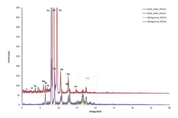
**FIG. 122** EDXRF spectra on White pigment: total spectra from different set-up, not subtracting background. Experimental set up: voltage 50 KeV and current 700  $\mu$ A, voltage 30 KeV and current 1300  $\mu$ A. Live time: 60 s, no filter, Helium flow, Anode Molybdenum, collimator 0.200
