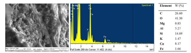
FIG. 129 SEM/EDS analysis on the backside of investigated white sample.
