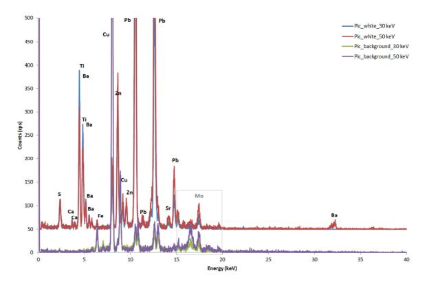
FIG. 56 XRF spectra on white pigment: total spectra from different set-up, not subtracting background. Experimental set up: voltage 50 KeV and current 700  $\mu$ A, voltage 30 KeV and current 1300  $\mu$ A. Live time: 60 s, no filter, Helium flow, Anode Molybdenum, collimator 0.200
