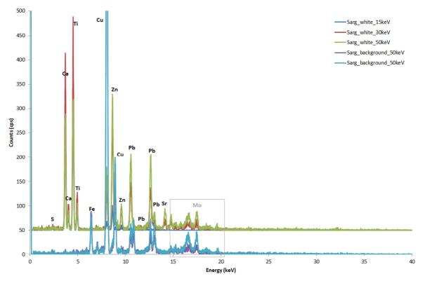
FIG. 39 XRF spectra on White pigment: total spectra from different set-up, not subtracting background. Experimental set up: voltage 50 KeV and current 700  $\mu$ A, voltage 30 KeV and current 1300  $\mu$ A, 15 KeV and 1500  $\mu$ A current. Live time: 120 s, no filter, Anode Molybdenum, collimator 0.650.
