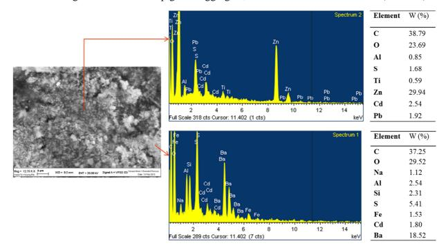
FIG. 128 SEM/EDS analysis on white sample: spectrum 1, aggregate of White Zinc oxide; spectrum 2, aggregate enriched in White Barium sulfate pigment.
