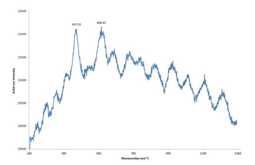
FIG. 45 Raman spectra on white samples (632,81 nm excitation, 50 x magnification): Rutile phase.
