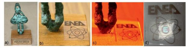
**FIG. 2** LiF-EUV tested on a copy of an archaeological bronze statue, known as "Hero four-eyes and four-arms": a) object with wooden base; b) adhesive tag under normal illumination; c) letter "E" patterned with EUV source appears in the centre of label using specific reading technique; d) LiF-EUV letter "E" is visible under normal light after attempt to remove it from an original item and to replace onto another (Bollanti S. et al., 2012).
